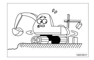
When using the machine as breaker or working in a place where stones may fall down, cab roof guard and head guard should be provided for proper protection.
